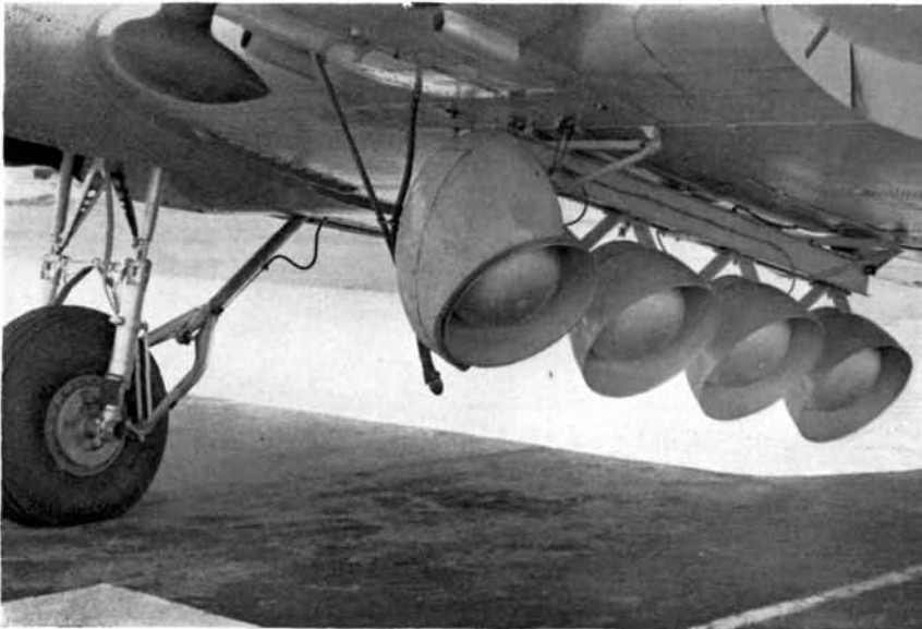
The four speakers are shown slung beneath the aircraft.
