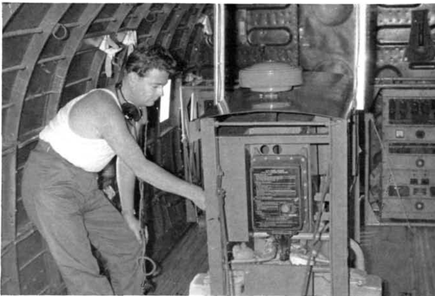
Inside the Dakota, setting the power supply from the diesel generator during ground test, is Cpl. A. D. Crowley.
